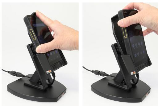
3. To remove the device from the holder: Place your index finger on the upper part of the holder and push at the same time as you pull the upper part of the device out from the holder. When the device is set free, lift it upward out of the holder.
