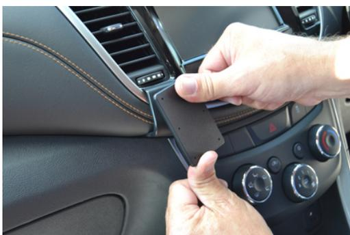
2. Rotate the ProClip upward so the angled edge on the lower part hooks behind the lower dashboard section. Press upward on the ProClip and hook the upper angled edge over the frame surrounding the air vent.
