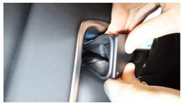
1. Use the enclosed alcohol pad to clean the area where the mount will be installed. Peel off the adhesive tape cover. Hook the angled lower edge of the mount behind the inner heardrest panel.
